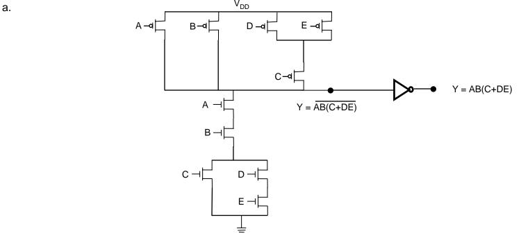
b.  $t_{pHL} = 0.69 R_{eq,n} (50e-15)$ . For worst case, we pull down through 4 NMOS transistors in series.  $R_{eq,n} = 4 (8.67 \text{ k}\Omega) = 34.68 \text{ k}\Omega$ . So  $[t_{pHL} = 0.69 (34.68e3) (50e-15) = 1.20 \text{ ns}]$ .  $t_{pHL} = 0.69 R_{eq,p} (50e-15)$ . For worst case, we pull up through 2 PMOS transistors in series.  $R_{eq,p} = 2 (20.67 \text{ k}\Omega) = 41.34 \text{ k}\Omega$ . So  $[t_{pLH} = 0.69 (41.34e3) (50e-15) = 1.43 \text{ ns}.$
